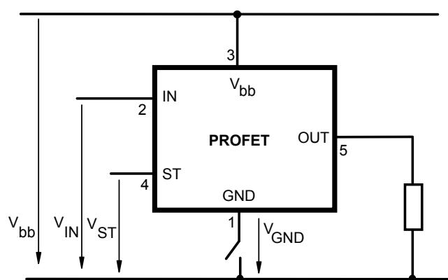
Any kind of load. In case of Input=high is  $V_{OUT} \approx V_{IN} - V_{IN(T^+)}$ .
