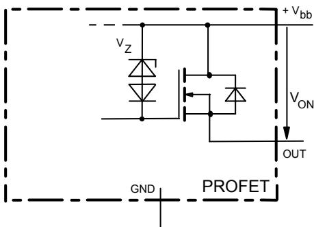
$V_{ON}$  clamped to 47 V typ.
