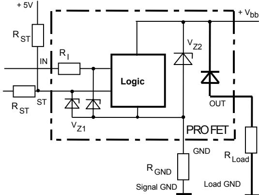
$$V_{Z1} = 6.1 \text{ V typ., } V_{Z2} = 47 \text{ V typ., } R_{GND} = 150 \Omega, \\ R_{ST} = 15 \text{ k}\Omega, R_l = 3.5 \text{ k}\Omega \text{ typ.}$$
