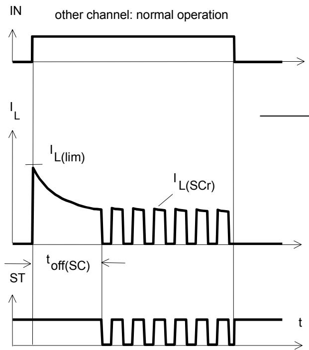
Heating up of the chip may require several milliseconds, depending on external conditions
